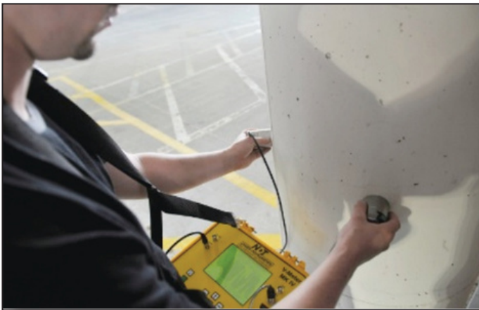
V-Meter MK IV evaluating a round column
